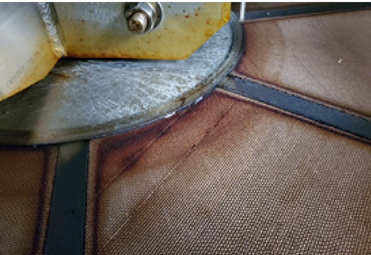
Above: Zeolite wheel surface coated with lacquer (yellow tint) from paint being drawn into the system.
