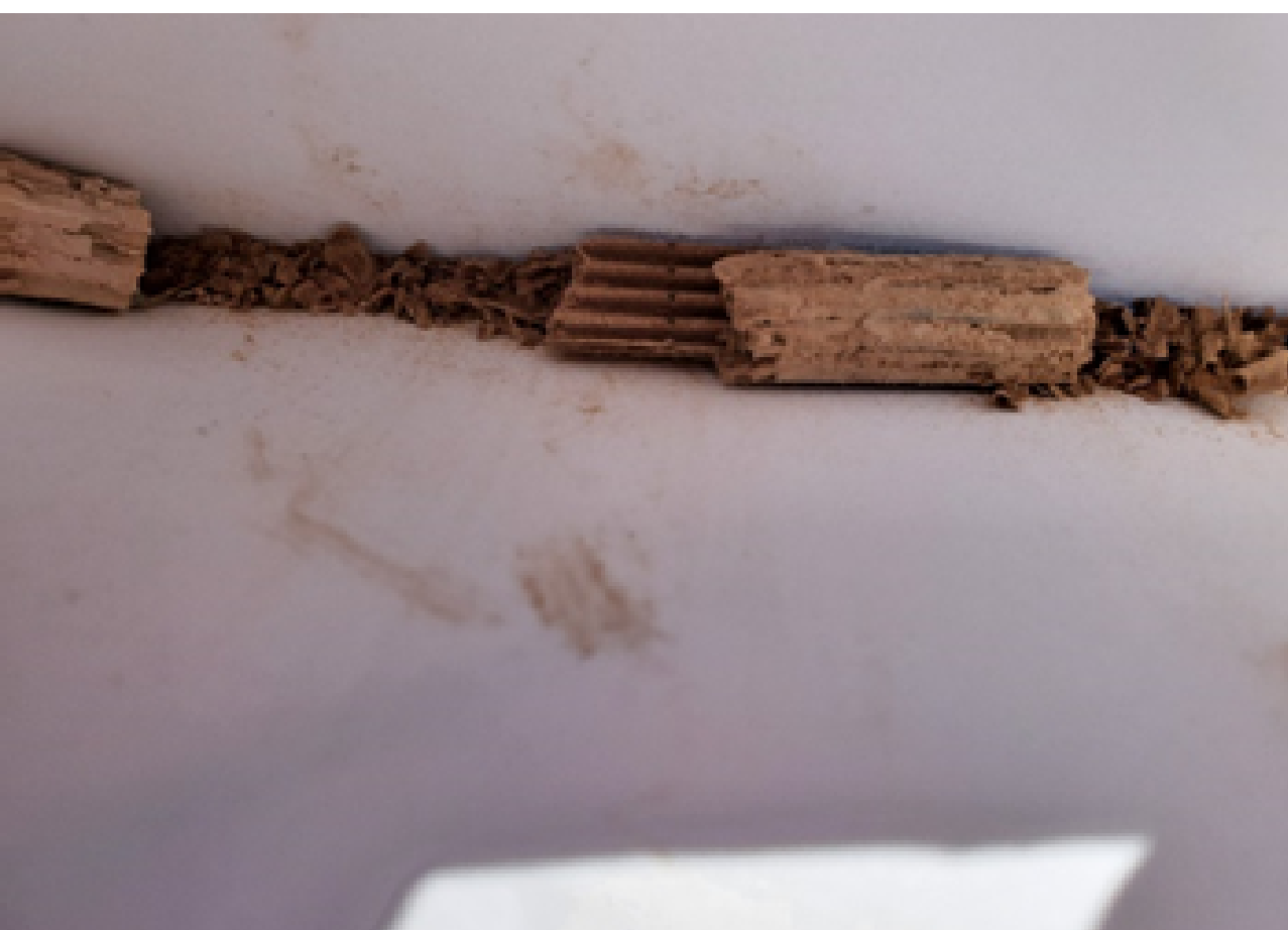
Below: Disintegrated core sample from wheel.
