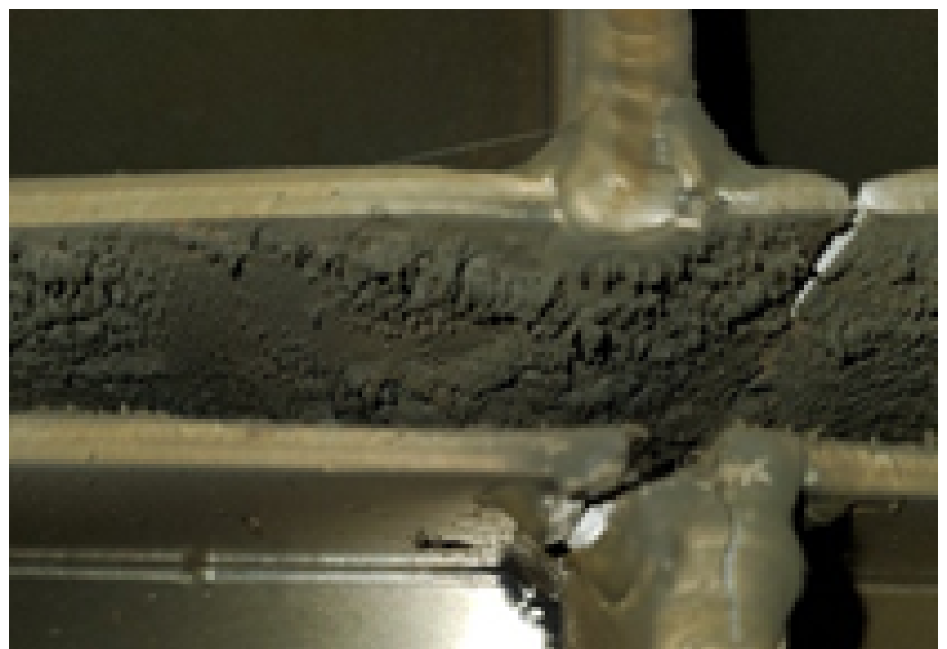
Below: Cracked baghouse filter frame
