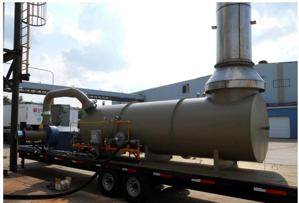
This oxidizer is designed to operate completely independent of the process and is equipped with an enable-disable signal interface in the system control panel.
