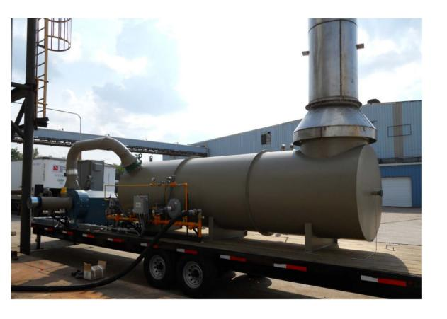
This oxidizer is designed to operate completely independent of the process and is equipped with an enable-disable signal interface in the system control panel.
